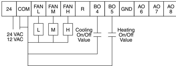
Fan Coil Wiring
