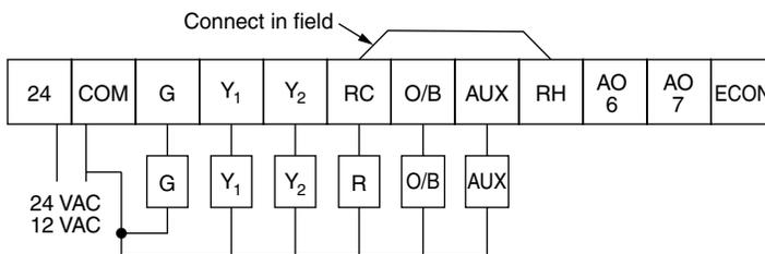
Heat Pump Wiring
